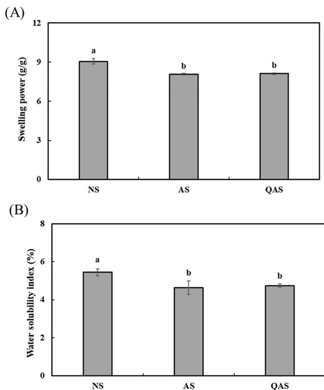
Fig. 4. Swelling power (A) and water solubility index (B) of native wheat starch (NS), annealed wheat starch (AS), and quercetin (QUE)-loaded annealed wheat starch (AS) (QAS). <sup>a,b</sup> Different letters represent significantly different from each other.
