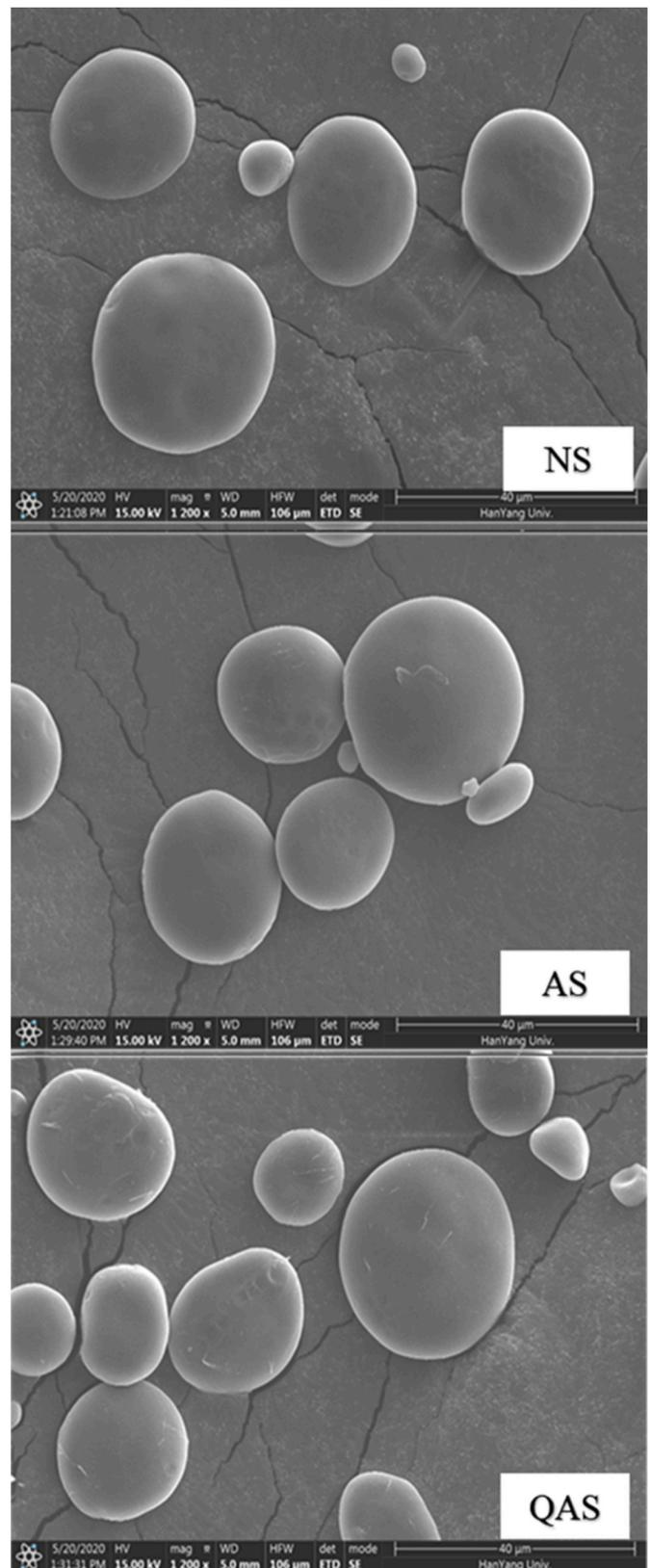
Fig. 2. Morphology of native wheat starch (NS) and annealed wheat starch (AS), and quercetin (QUE)-loaded annealed wheat starch (AS) (QAS).
